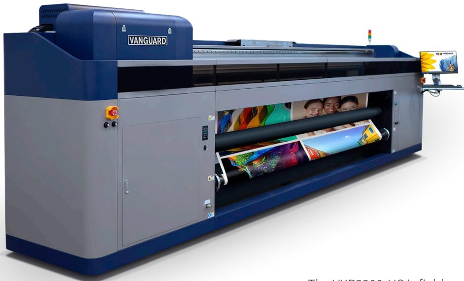
The KJ4A is a dual channel printhead design that supports two colors at a time. The small 4 picoliter drop size ensures tight dot placement for a vividly printed output on flexible substrates up to 1” thick. These advanced features make it the fastest and most accurate printer in its class.
